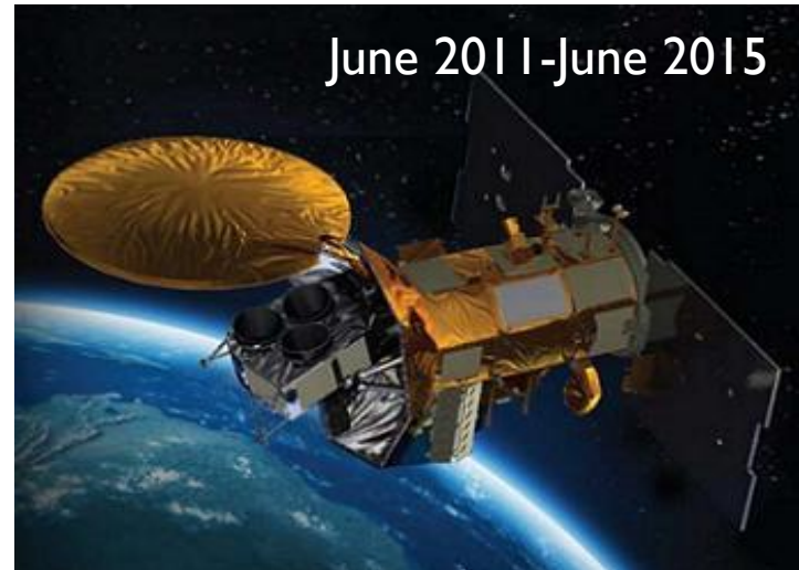
Aquarius/SAC-D Mission by NASA & CONAE L-band radiometer + radar
