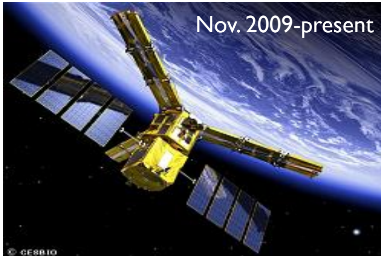
Soil Moisture & Ocean Salinity (SMOS) Mission by European Space Agency L-band radiometer
