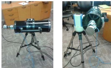
Figure 6: State of the Art polarimeter with automation in collaboration with L-1 Standards and Technology LLC., which enables polarization measurements of the moon, atmosphere and surfaces. (To be tested at UMD Observatory)
