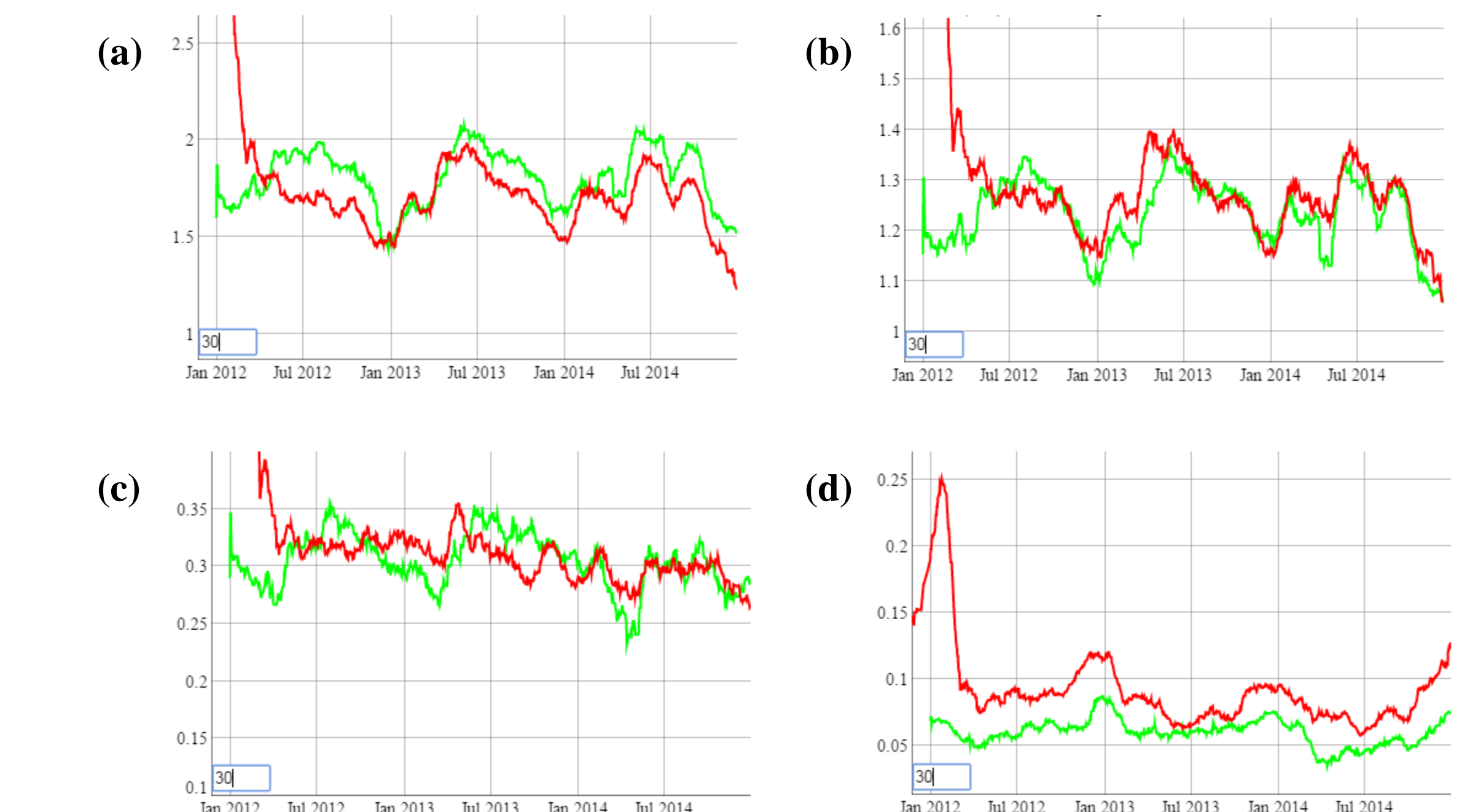
Fig. 5. Time series of reprocessed VIIRS ocean color EDR data (red) compared with those of MODIS-Aqua (green) (30-day running means) at around MOBY location for (a) nL w (443), (b) nL w (486), (c) nL w (551) (unit: mW cm -2 μm -1 sr -1 ) and (d) Chl-a concentration (unit: mg m -3 ).
