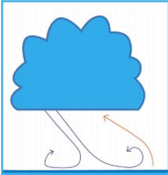
Figure 2-9a. Cross section of flow associated with a sheared convective cloud (blue). Vertical wind shear is from left to right (i.e. the synoptic scale wind is from left to right and increasing with height). Convective downdraft is depicted by blue arrows and convective updraft is depicted by a red arrow.
