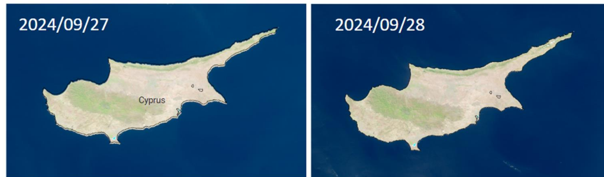
Alignment of Suomi NPP VIIRS SDR projected image with the Cyprus coastline before (left) and after (right) recovery from the spacecraft GPS anomaly on 9/24/2024: the geolocation errors are still visible on 9/27/2024 before the GPS reset at ~16:34 UTC
