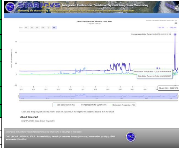
(a) S-NPP ATMS scan drive main motor current in vector display page
