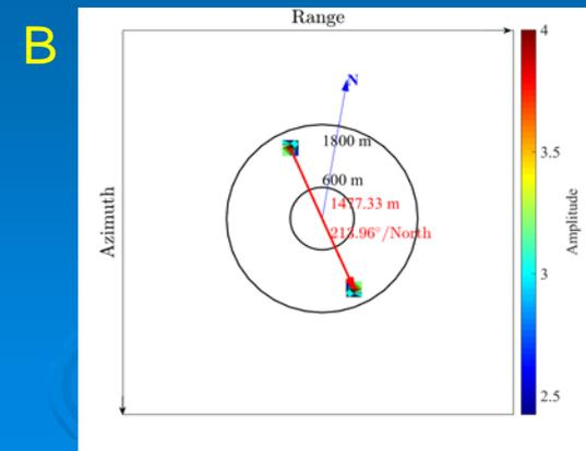
Two dimensional FFT analysis of SAR image shows the dominant wavelength and orientation of the boundary layer rolls with 180 degree ambiguity.
