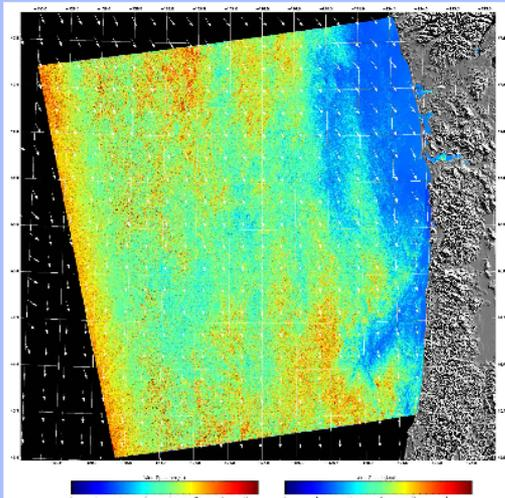
A color-coded sea surface wind speed image retrieved from RADARSAT-1 SAR overlaid with QuikSCAT scatterometer wind vectors of the U.S. west coast.
