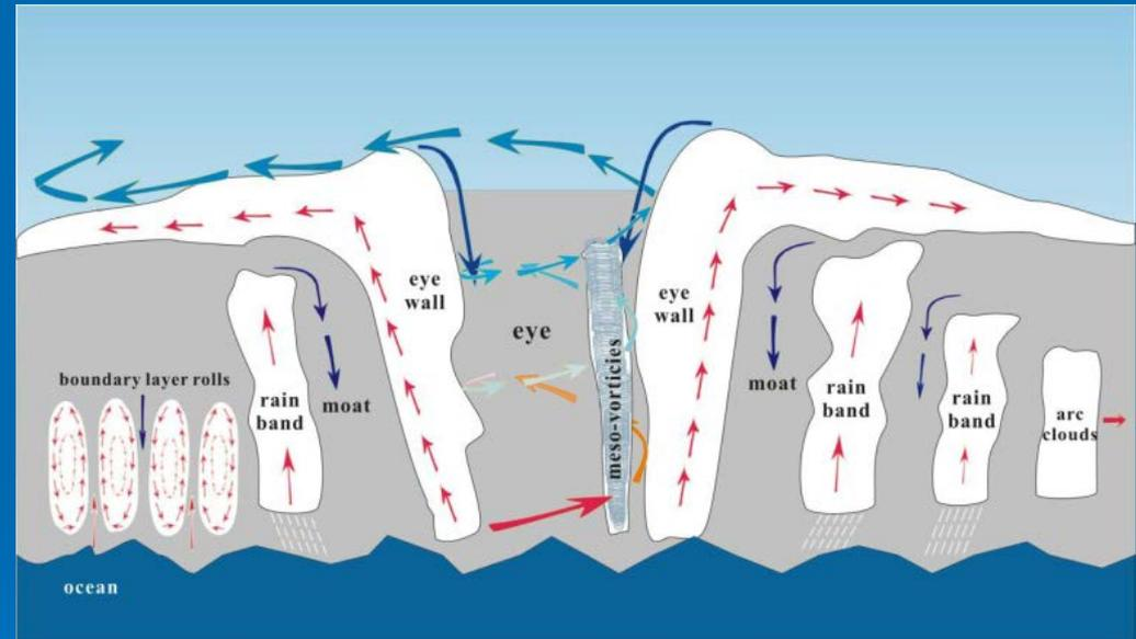
Schematic plot of tropical cyclone structure and atmospheric phenomena including eye/eyewall, rain band, boundary layer rolls, arc cloud, and meso-vortices (not to scale).
