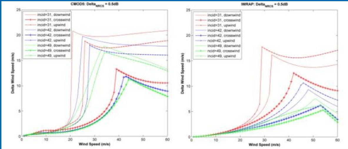
Wind retrieval errors due to NRCS calibration errors
