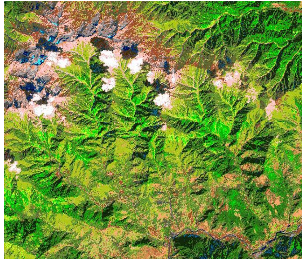
Fig. D. Zoomed area extracted from the 45-class output map shown in Fig. B. Adopted pseudo colors are the following. Green tones: vegetation and rangeland, Brown and grey color shades: barren land and built-up areas, Blue tones: water types, White tones: clouds, Light blue tones: snow and ice, etc.
