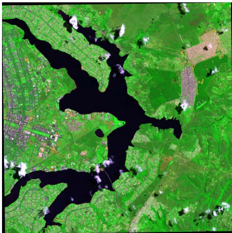
Fig. A. 8-band WorldView-2 VHR image of the city of Brazilia, Brazil, acquired on 2010-03-16, at 13:25 p.m., depicted in false colors (R: band R, G: band NIR1; B: band B) (provided by DigitalGlobe, 8-Band Challenge), calibrated into TOA reflectance. Spatial resolution: 2.4 m.
