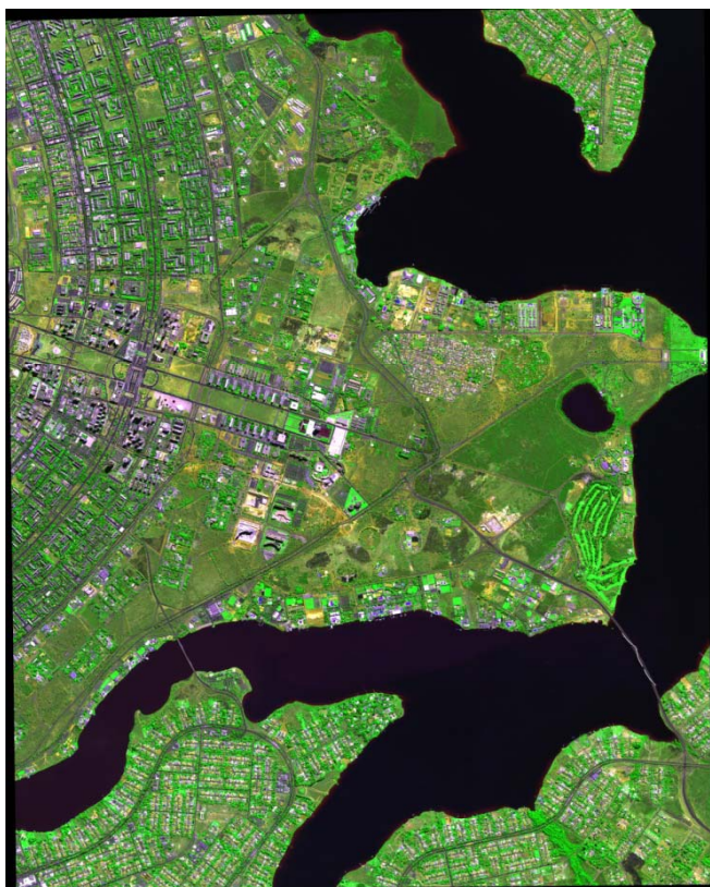
Fig. A. 8-band WorldView-2 VHR image of the city of Brazilia, Brazil, acquired on 2010-08-04, at 13:32 p.m., depicted in false colors (R: band R, G: band NIR1; B: band B) (provided by DigitalGlobe, 8-Band Challenge), calibrated into TOA reflectance. Spatial resolution: 2.0 m.
