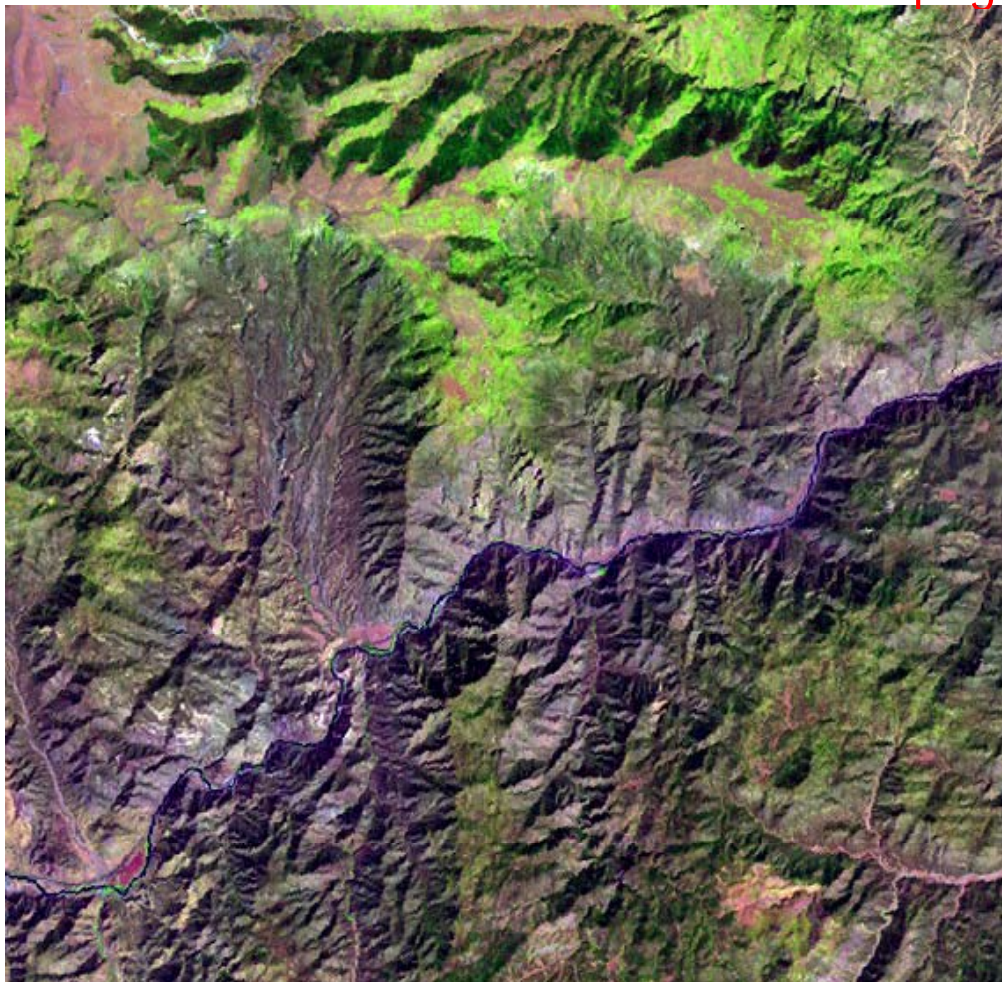
Fig. A. Zoomed area of a Landsat 7 ETM+ image of Colorado, USA (path: 128, row: 021, acquisition date: 2000-08-09), depicted in false colors (R: band ETM5, G: band ETM4, B: band ETM1), 30m resolution, calibrated into TOA reflectance.
