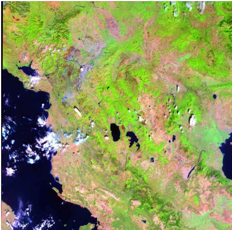
Fig. A. IRS-P6 AWiFS Image acquired on Sept., 2007, covering a surface area in Greece (R: band 4, G: band 3, B: band 1), spatial resolution: 56 m.
