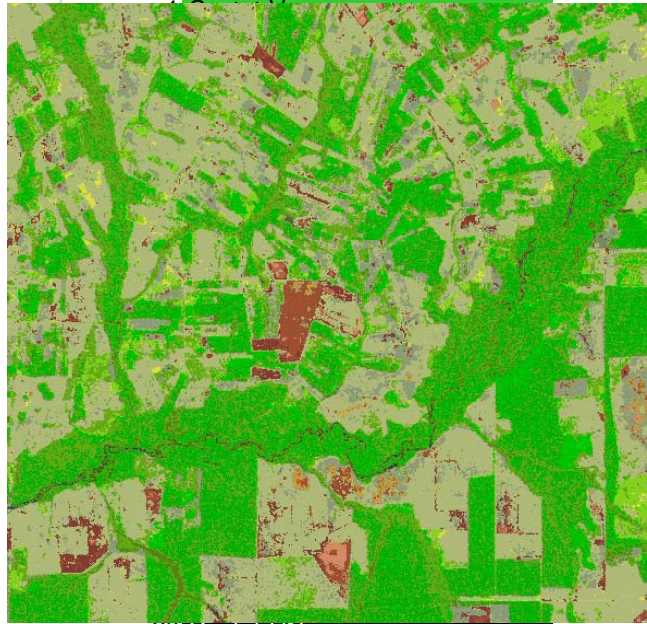
Fig. B. Zoom of a preliminary classification map depicted in pseudo colors, generated from a Landsat-5 TM imagery acquired on 2006-07-16, covering an area of Brazil (path: 231, row: 068), spatial resolution: 30 m.
