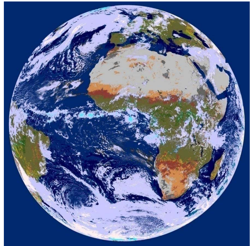
Fig. B. Output map generated from Fig. A, consisting of 49 spectral categories. Adopted pseudo colors are the following. Green tones: vegetation and rangeland, Brown and grey color shades: barren land and built-up areas, Blue tones: water types, White and light blue: cloud types, etc.
