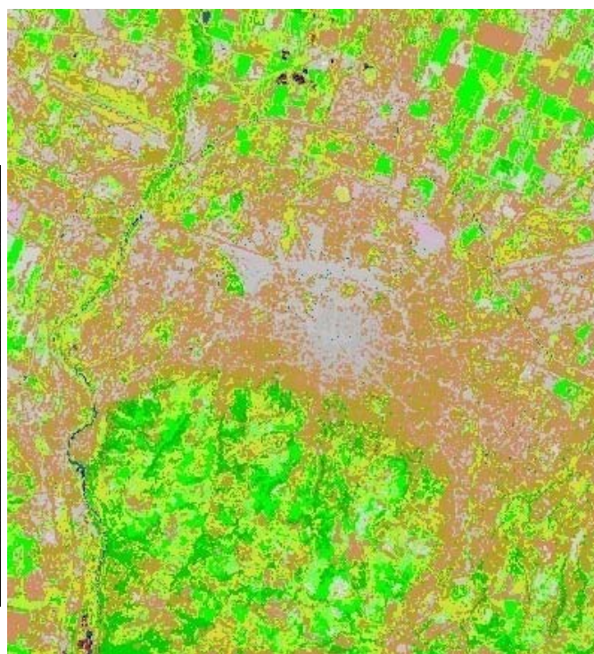
Fig. B. Output map generated from Fig. A, consisting of 31 spectral categories. Adopted pseudo colors are the following. Green tones: vegetation and rangeland, Brown and grey color shades: barren land and built-up areas, Blue tones: water types.
