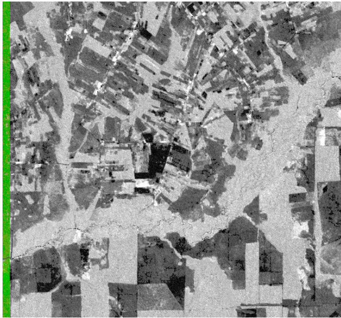
Fig. A. Zoom of a preliminary classification map depicted in pseudo colors, generated from a Landsat-5 TM imagery (acquired on 1985-08-16, covering an area of Brazil (path: 231, row: 068), spatial resolution: 30 m).
