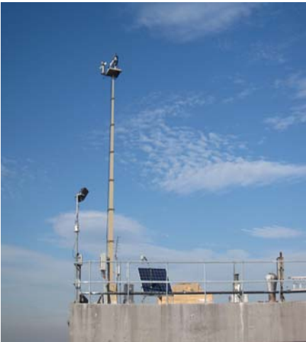
Fig 1 SeaPRISM and HyperSAS on the tower
