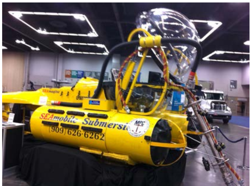
This SEAmobile Submersible, on display at IOSC 2011, acts like an underwater helicopter for detecting oil spills in the ocean. Credit: NOAA
