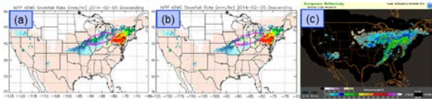
Figure 12. SFR product from a snowstorm on Feb 5, 2014 using (a) the newly developed combined SD algorithm, and (b) the previous single-module SD algorithm. Image (c) is the coincident composite NEXRAD reflectivity.
