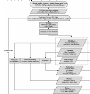
Schematic representation of gridding and analysis of gridded data in Global QC/QA Tool (GQT) . Anomaly maps and trend-plots (bias vs. correlating variables, e.g. zenith angle) are major outputs of the gridded level processing.
