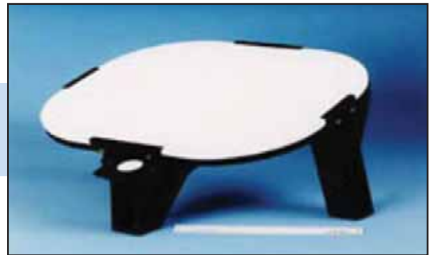
Figure 8 Picture of the MODIS Solar Diffuser from modis.gsfc.nasa.gov/about/soldiff.php
