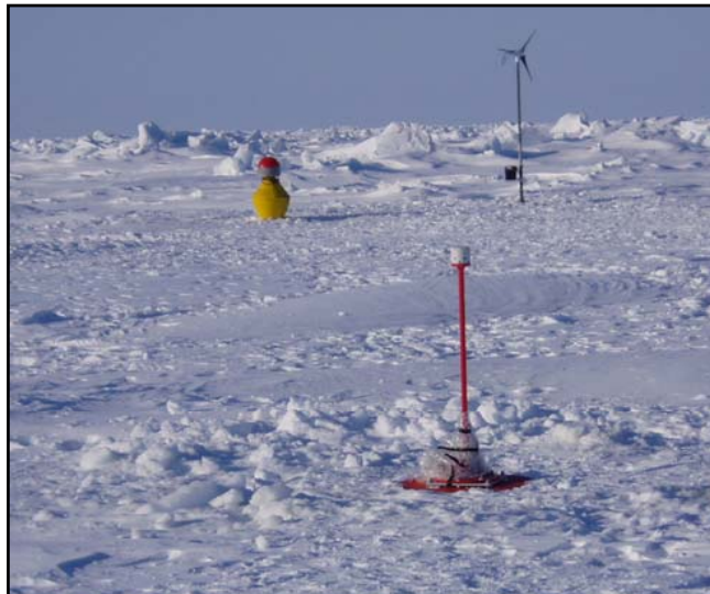
Polar Ocean Profiling System (foreground) & Ocean Flux buoy (yellow) Monitors Air and Ocean (typically deployed with IMB buoys)
