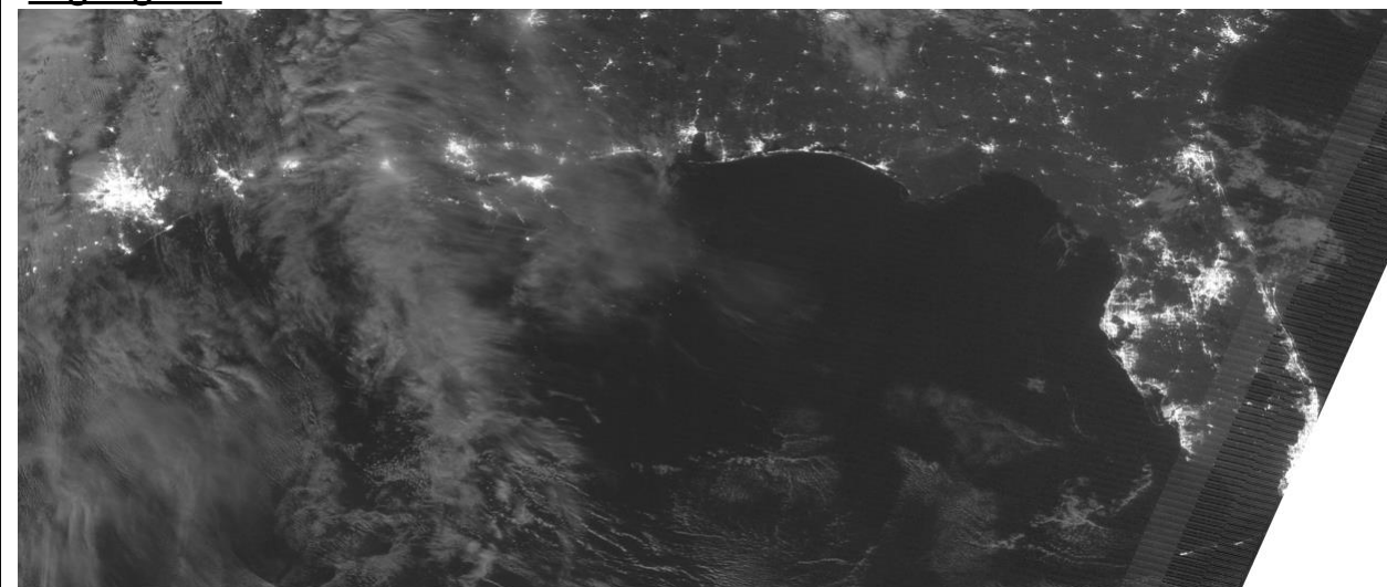
Suomi NPP VIIRS DNB re-projected image acquired after recovery from the SBC Lockup anomaly on 4/24/2024: striping visible along the edge on the right side
