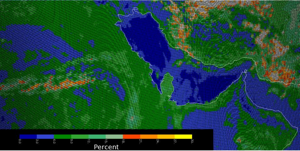
This image shows the effective reflectivity for the 380-nm Channel for part of an orbit of small Fieldof-View (5 KM X 10 KM at Nadir) made by the OMPS Nadir Mapper in a special diagnostic mode. The Qatar peninsula sticking into the Persian Gulf in the middle of the picture lies along the nadir view of the orbital track and gives a preliminary assurance of the geolocation at better the 5 KM.
