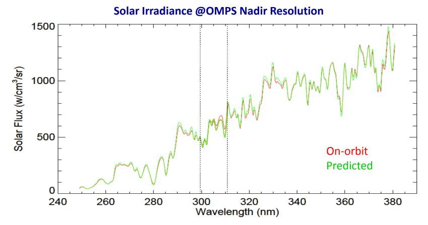
Observed solar irradiance is within ~2% of predicted synthetic solar spectra:
