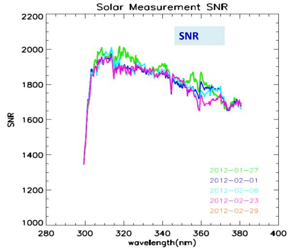
Solar measurement SNR meets the system requirement of 1000
