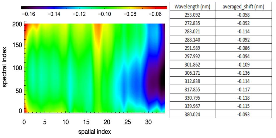
Wavelength changed less than 0.16 nm from ground to orbit.
